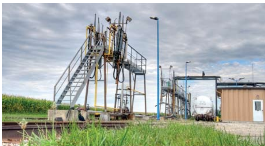
Rail tankcars can be loaded and unloaded at the Van Wert terminal. The loading racks provide access to railcars on both sections of track at the terminal.
