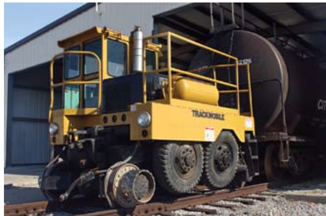
Workers at the Morrystown site use this Trackmobile unit to reposition rail tankcars at the facility.
