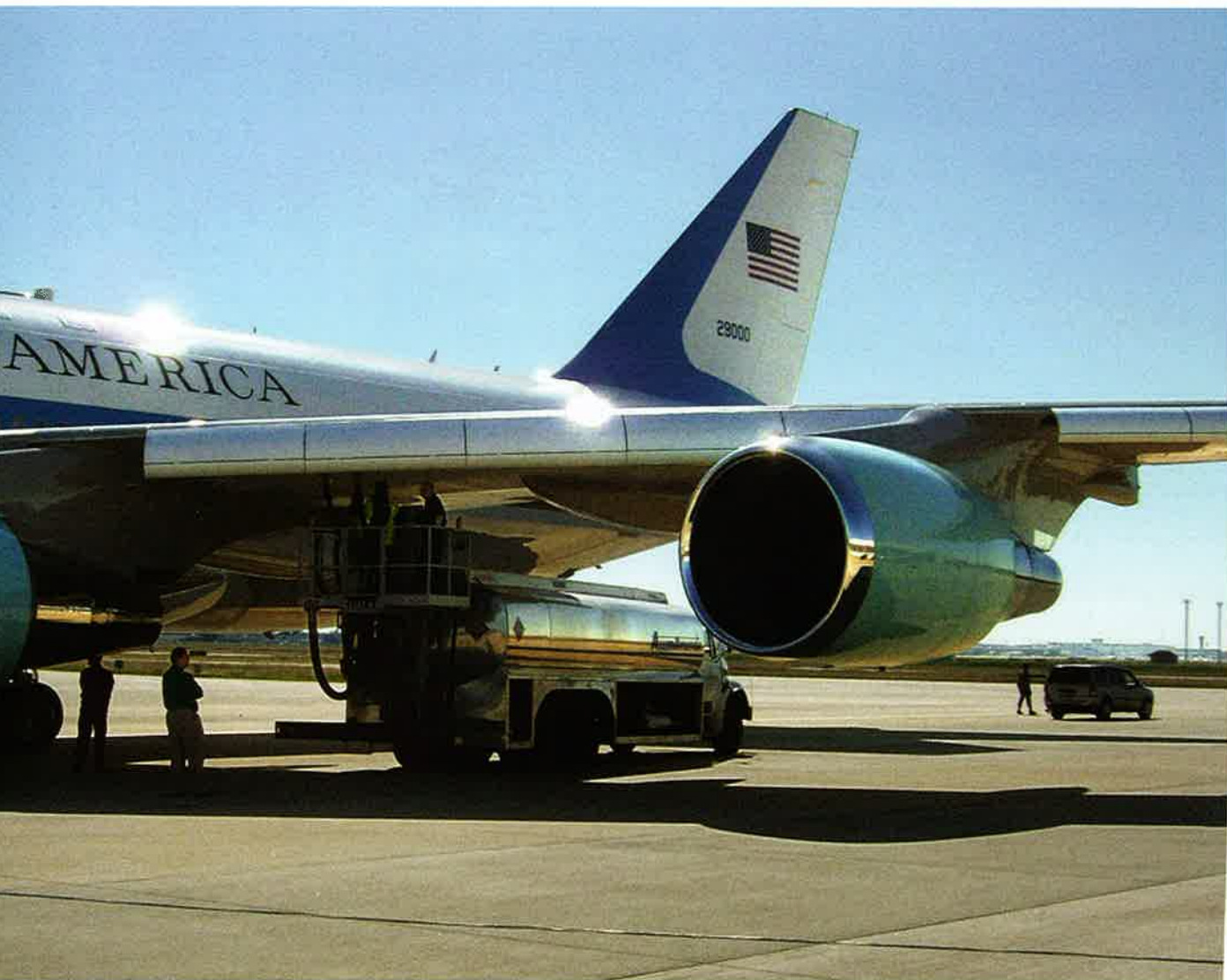
Allied Aviation personnel refuel Air Force One at Houston's George Bush Intercontinental Airport (IAH). The refueling service provider handles more than 1.5 million gallons of Jet A fuel every day at IAH. The company manages the entire fuel distribution system at the airport.
