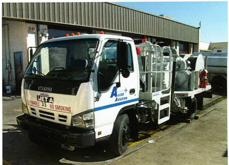
Hydrant trucks, like this unit on an Isuzu chassis, handle a majority of the refueling duties at IAH. Hydrant carts also are used in the operation.
