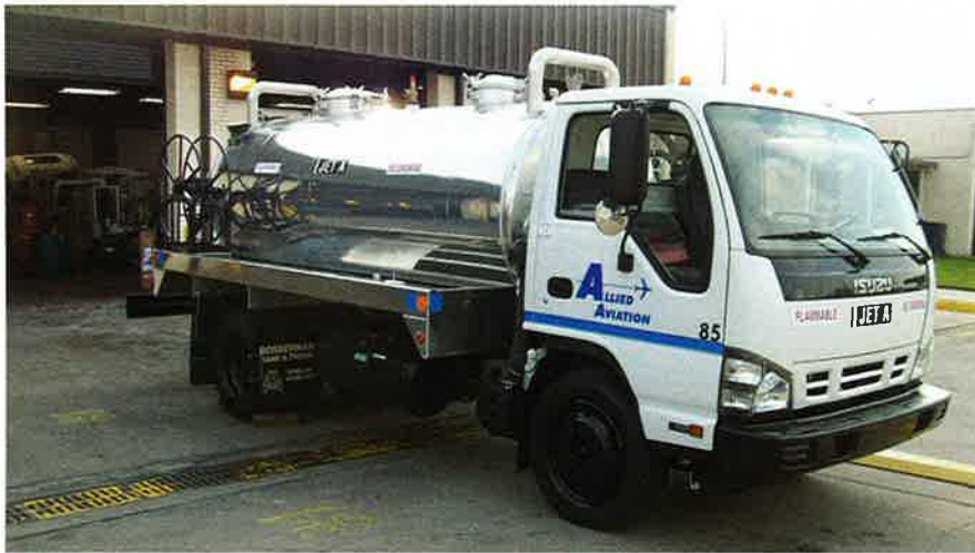
Tanker units called sump trucks are used to vacuum out the hydrant sumps when the in-ground fuel distribution system is serviced at IAH. Mounted on the trucks are non-code vacuum tanks with capacities ranging from 800 to 1,500 gallons.
