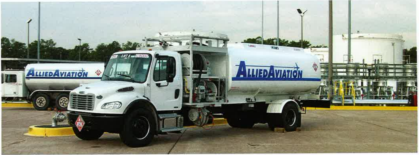
A variety of refueler trucks are part of the Allied Aviation fleet at IAH. This unit on a Freightliner Business Class chassis is one of the newest refuelers in the Houston operation. Cargo tank capacities range from 3,000 to 10,000 gallons. Refuelers have non-code cargo tanks.
